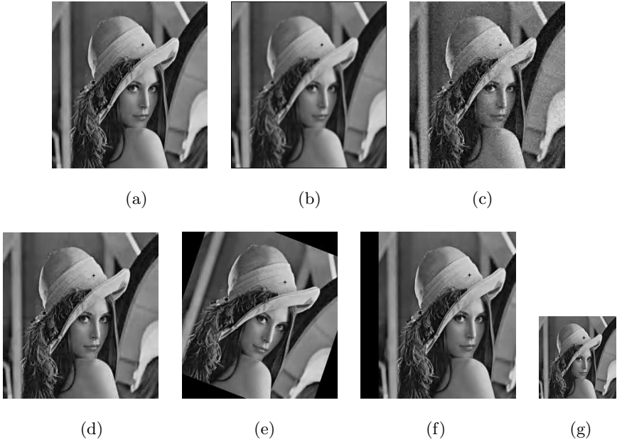
Fig. 5. Invariant centroids which are marked as cross: (a) original image; (b) 3 \times 3 average filtered; (c) 5% gaussian noise added; (d) JPEG compressed image with compression ratio of 70; (e) 20 degree clockwise rotation of image plus cropping; (f) 30 pixels translated along x axis; (g) scaled image based on scaling factor of 0.5.
